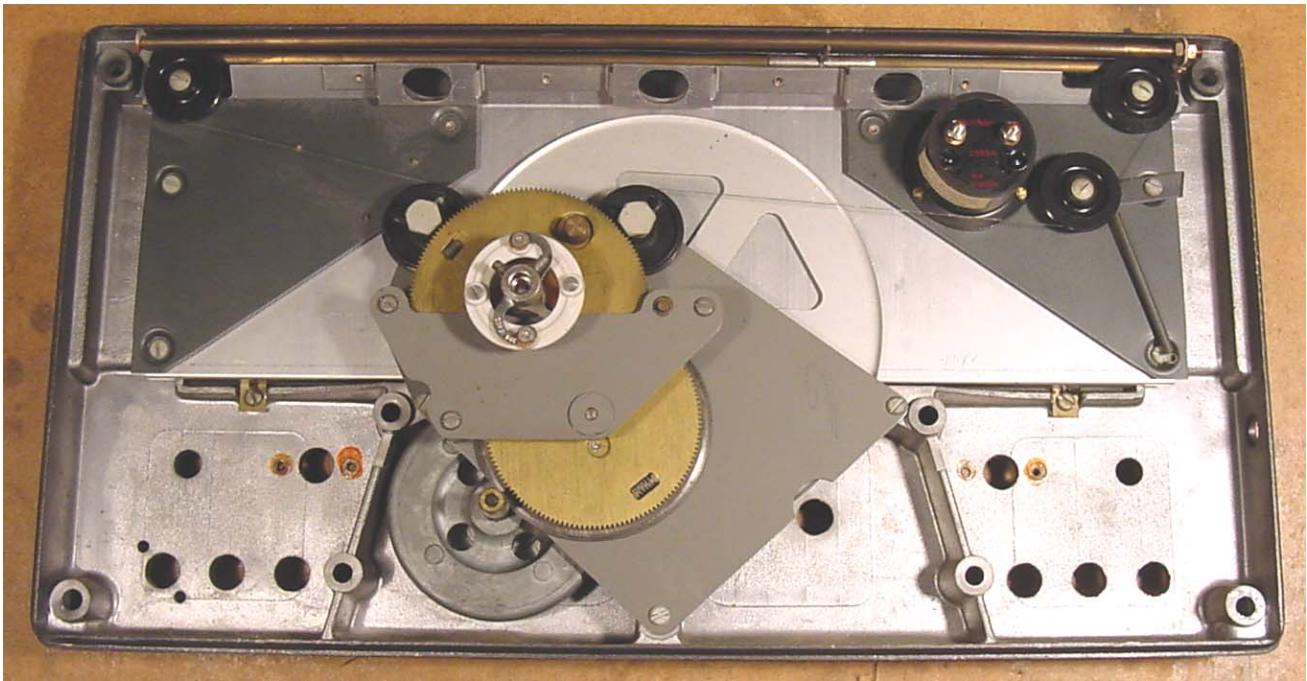
Above: Late-model S.680X front panel and gearbox. Below: S.680/2 front panel and gearbox. This is the most radically-changed part of the set. Note the difference in location of the tuning shaft coupling
